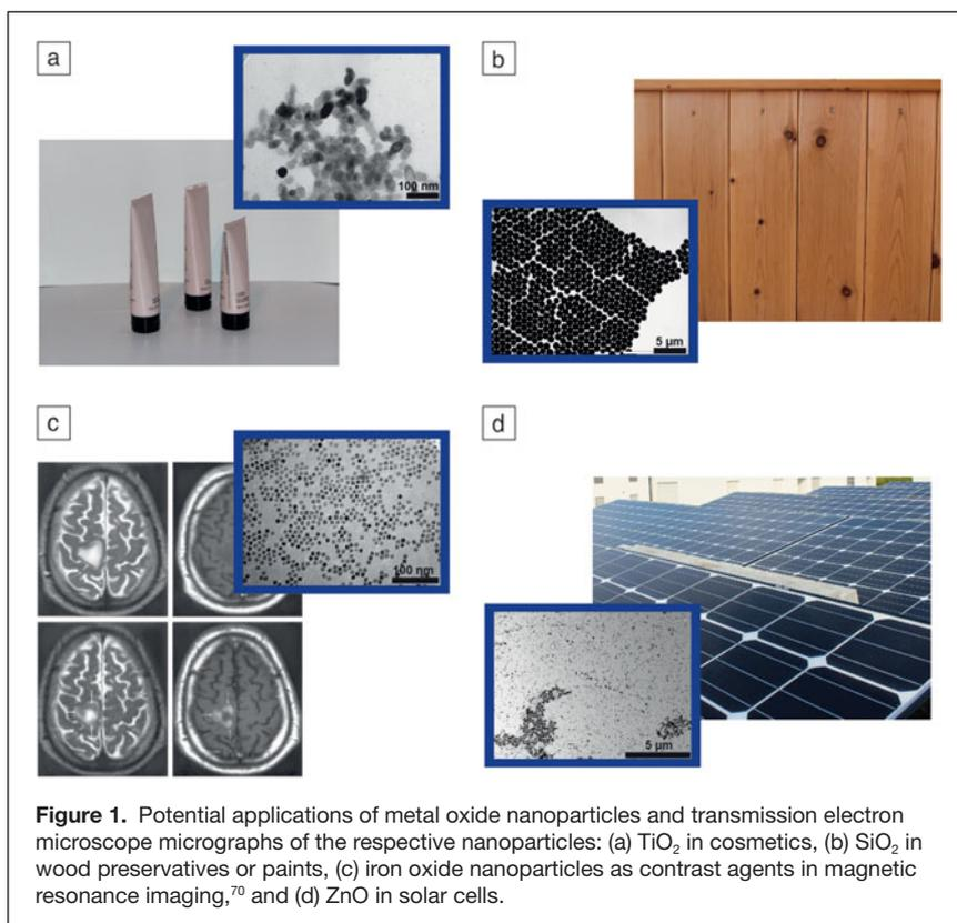
**Figure 1.** Potential applications of metal oxide nanoparticles and transmission electron microscope micrographs of the respective nanoparticles: (a)  $\text{TiO}_2$  in cosmetics, (b)  $\text{SiO}_2$  in wood preservatives or paints, (c) iron oxide nanoparticles as contrast agents in magnetic resonance imaging,<sup>70</sup> and (d)  $\text{ZnO}$  in solar cells.
