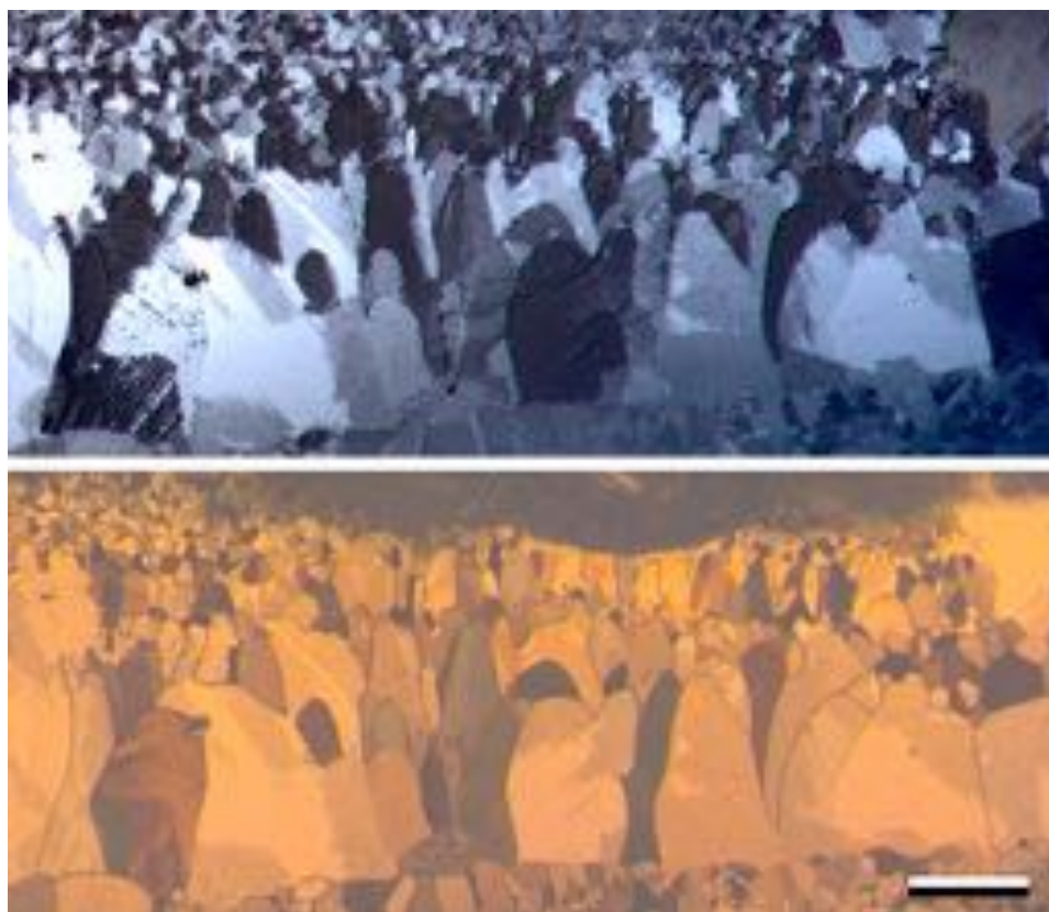
Figure 6.8. Domain pattern in polymer film and gold replicate. Optical micrographs of the as annealed polymer film (top) and a free-standing gold replicate (bottom) were recorded under crossed polarisation. Equivalent domain patterns are observed in both cases, which indicates a correlation between the alignment of the crystallites and the microphase separated geometry. The scale bar is 200 \mu\text{m} .
