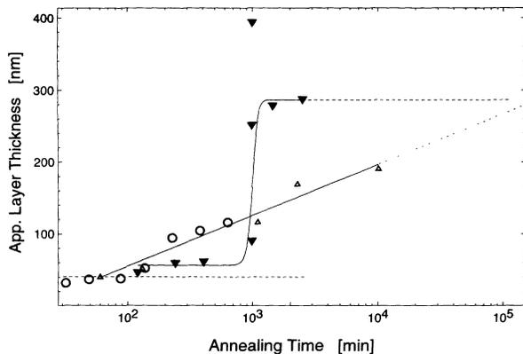
FIG. 4. Variation of the apparent thickness of the surface-preferred phase at the air surface with annealing times, on a semilogarithmic plot. Solid symbols ( $\blacktriangle$ ) are from the present study. The curve is a guide to the eye. The open symbols ( $\triangle, \circ$ ) are from a similar study using a different binary mixture [17], where the growth with time of the surface layer obeys a logarithmic variation, as also reported earlier for the case of complete wetting conditions [9].
